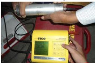
2. **Ultrasonic Pulse Velocity Test:** This test is performed by measuring the travel time of an ultrasonic pulse moving through the concrete being assessed. Higher velocity means better concrete quality.
