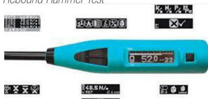
1. **Rebound Hammer Test (Schmidt Hammer):** This test is used to establish the concrete uniformity and delimit areas with low quality concrete. Also, this test is useful when detecting transitions or changes in the concrete behavior. The compression resistance of the concrete can also be established using empirical relations.
